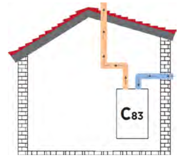
The boiler draws combustion air from outside via a separate supply pipe routed through the external wall, and expels flue gas to the outside via flue pipe leading through the roof.
